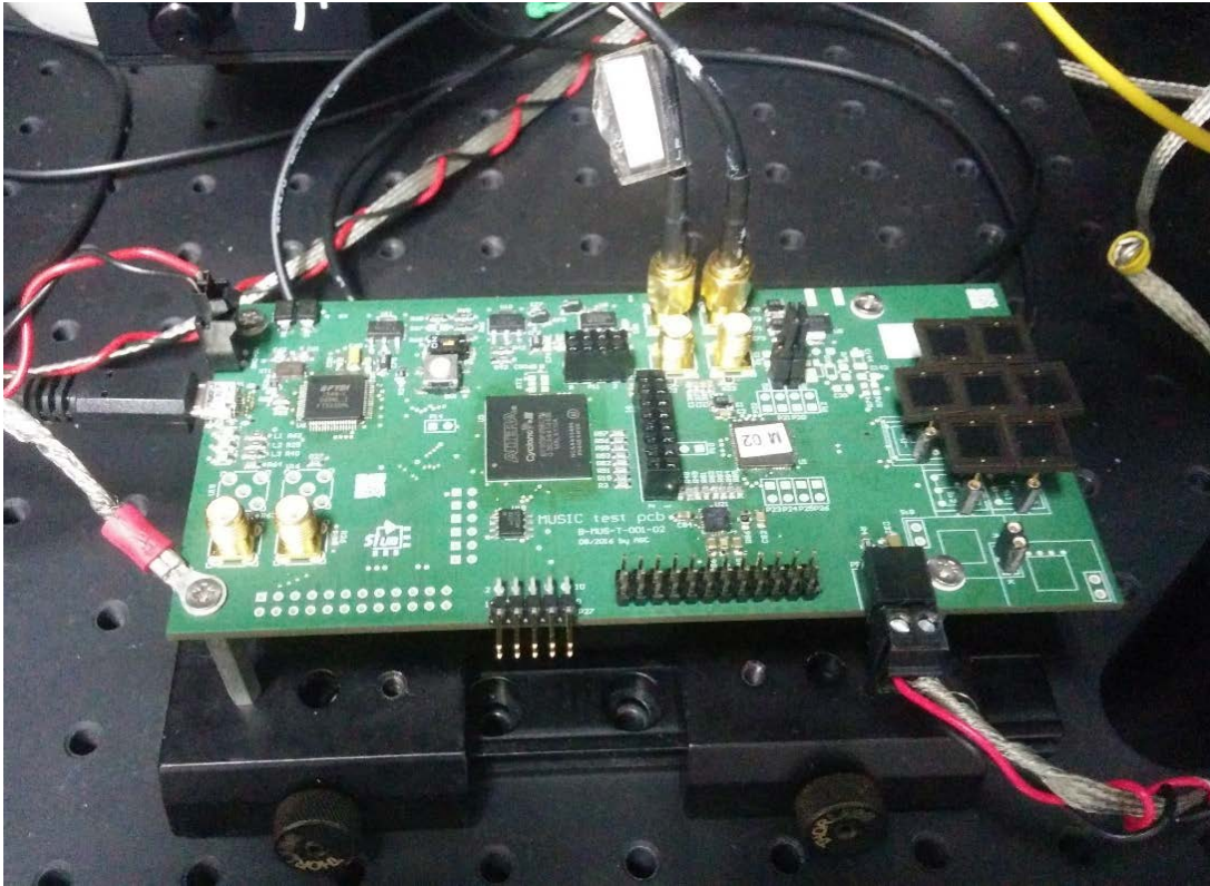
Figure 5: 7 SiPM matrix using the MUSIC board
