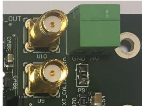
Figure 6: ·EXT_CALIB_VA_input and EXT_TRG_OUT SMA output.
