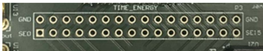
Figure 8: Socket access to measure TIME/Energy per channel.
